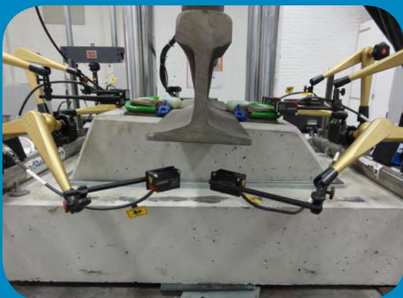
edilon)(sedra testing centre, using the new type of non-contact laser sensors
